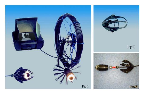
The Camera Reel (6mm & 7mm) is designed to allow the operator to inspect smaller chimneys and gas vents from below and from above as well as dryer vents, ducts and any other horizontal pipes and flues. The camera rod has the video electronics imbedded inside the rod. The transmission of the video signal from the rotating rod through the non-rotating Monitor connection is through a patented central hub.
