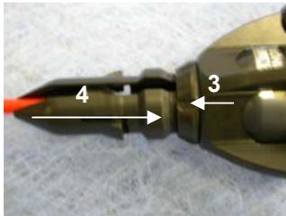
To connect the P&T Camera head to the 6mm or 7mm Video rods with the camera roller:
